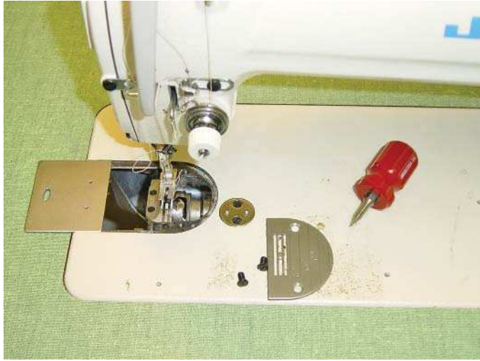
Photograph 3 Throat Plate Removed
