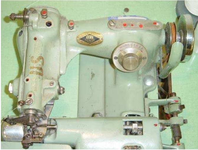
Photograph 5 Blind Hemmer with Oiling Holes Marked
